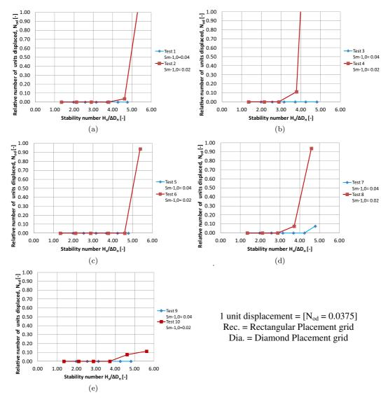
Fig. 8.  $N_{\rm od}$  versus stability number  $(H_s/\Delta D_n)$  for all tests- (a) Rec. grid with  $\phi = 0.69$ , (b) Dia. grid with  $\phi = 0.63$ , (c) Rec. grid with  $\phi = 0.66$ ; (d) Rec. grid with  $\phi = 0.63$  and (e)  $\phi = 0.66$  with higher crest freeboard ( $R_c = 0.185$ ).
