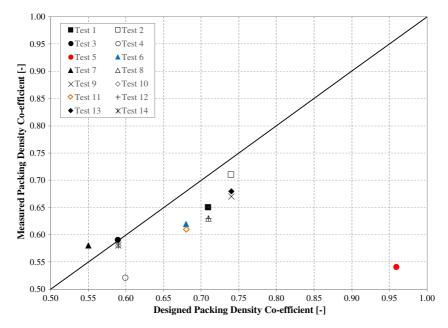
Fig. 7. Designed nominal packing density co-efficient against measured nominal packing density co-efficient.
