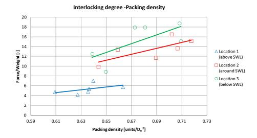
Fig. 16. Overview of interlocking degree corresponding to packing density after wave attack.
