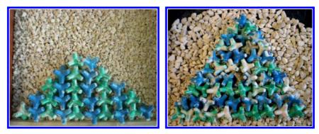
Uniform placement using smaller underlayer in a rectangular grid
