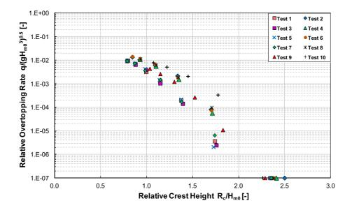
Fig. 9. Relative overtopping discharge as a function of relative freeboard.
