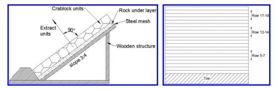
Fig. 5. Test set up of pull tests.
