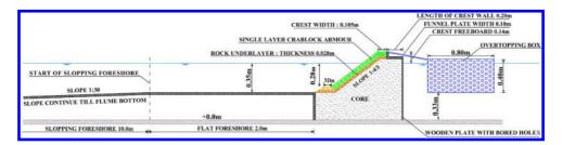
Fig. 4. Cross-section of breakwater with crest height  $1.2 \times H_{sD}$ ; tests 1–8.
