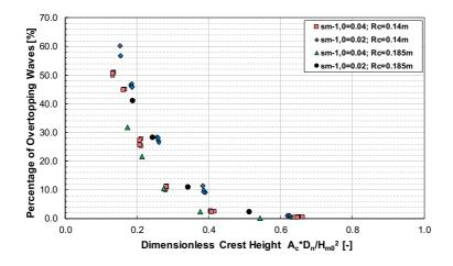
Fig. 11. Percentage of wave overtopping as a function of dimensionless crest freeboard.
