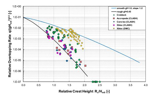
Fig. 10. Test results compared to empirical prediction and other monolayer units.
