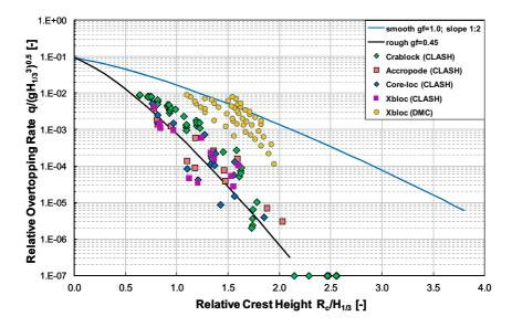
Fig. 13. Test results compared to empirical prediction and other monolayer units (using  $H_{1/3}$ ).
