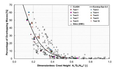
Fig. 12. Test results on percentage of overtopping compared to empirical prediction and other single layer units.
