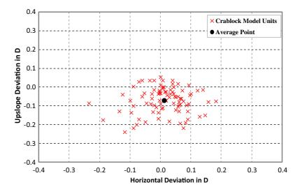
Fig. 6. Deviation of units from their intended position (Test 13).
